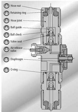
Generic Pump Schematic and Description of Parts
