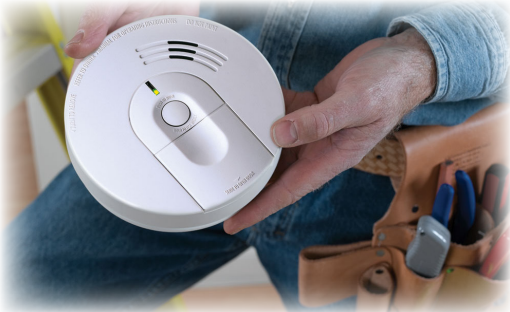
Install a smoke alarm on every level of the home and inside each sleeping area.
