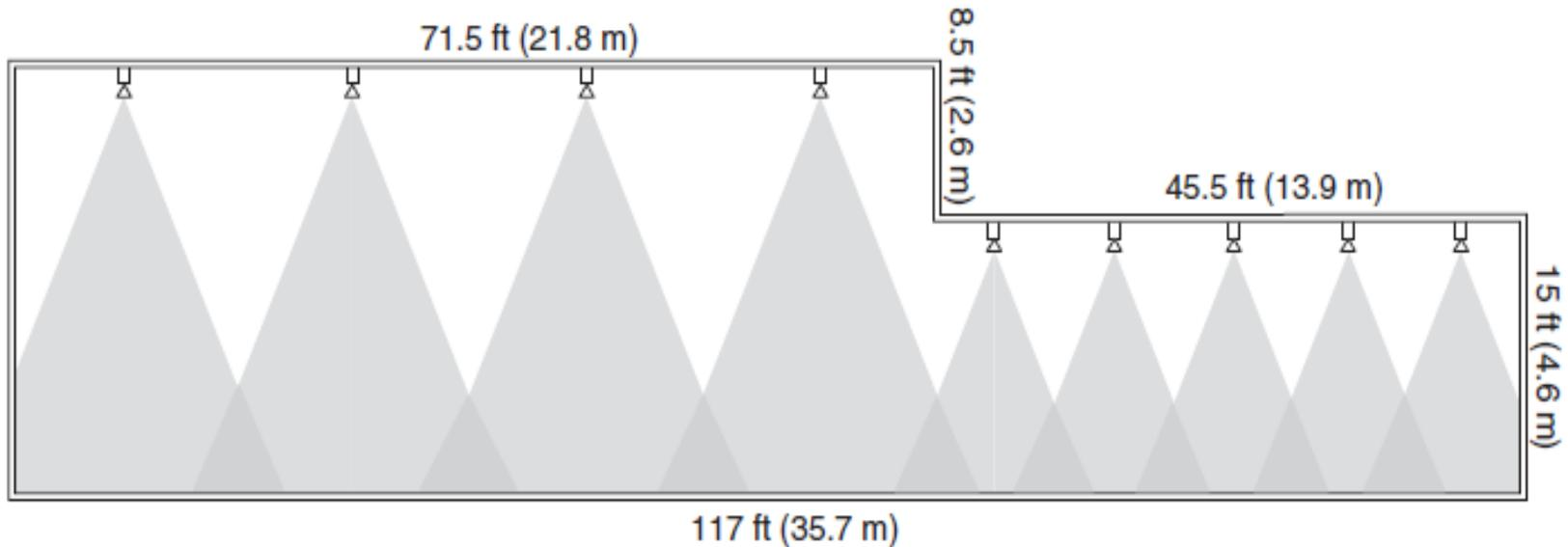
**FIGURE D.2.3.1.7** Illustration Demonstrating Effect of Ceiling Height. (Source: R. P. Schifiliti Associates, Inc.)
