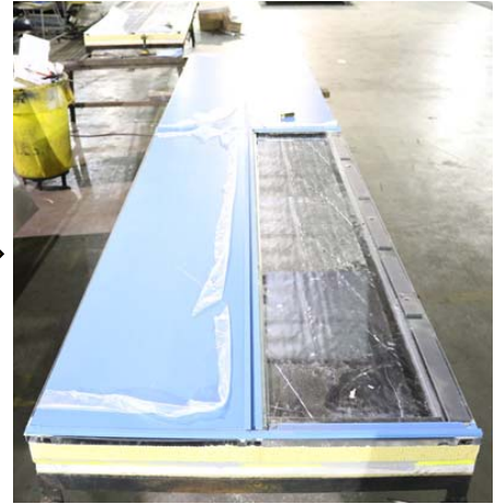
Joint system & ACMs with air cavity
