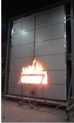
17 ft x 13 ft Propane line burners : 1300 kW
