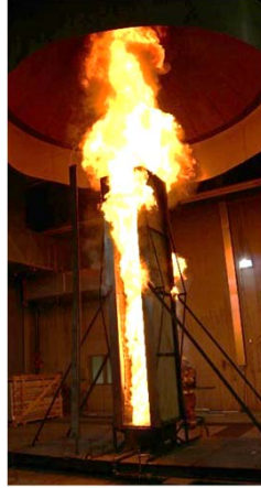
FM 16-ft Test #3 (Similar to Grenfell) Failed NFPA-285
