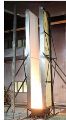
16 ft x 3.5 ft 360 kW Propane sand burner
