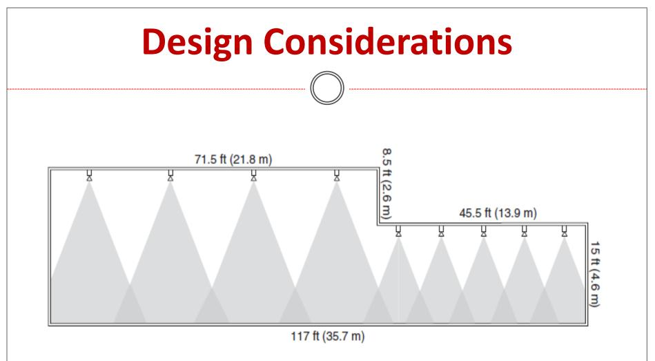
FIGURE D.2.3.1.7 Illustration Demonstrating Effect of Ceiling Height. (Source: R. P. Schifiliti Associates, Inc.)
